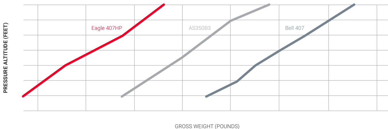
HOVER CEILING OUT OF GROUND EFFECT COMPARISON (20°C)
